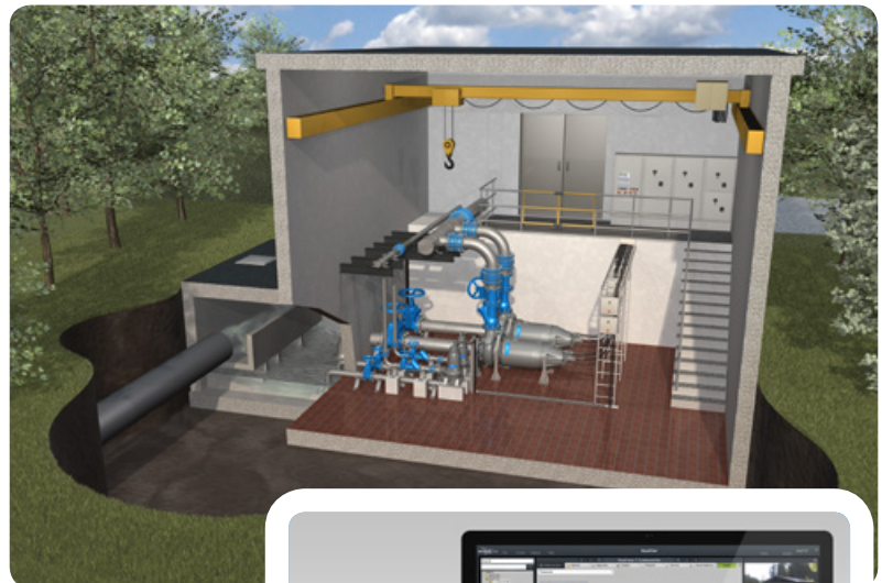
Dry-installed submersible pumps
